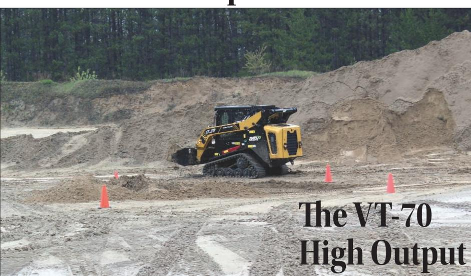
PHOTOS BY BRITTA ARENDT | HERALD-REVIEW Above, ASV's newest product, the VT-70 High Output Posi-Track machine was unveiled this week at the company's test track in Grand Rapids. The VT-70 features unmatched power, comfort, serviceability and speed for lift, carry and load tasks. It has an amplified level of torque and an efficient hydraulic system for operators to get maximum performance.
