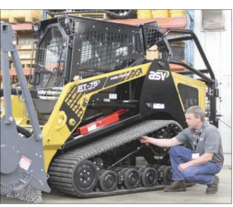
Above, Buck Storlie, ASV Product Line Manager, pointed out some of the features of ASV engineering before showcasing the new VT-70. This includes a specially-designed undercarriage with an all-rubber track system with torsion axle suspension that is very resistant to the elements.
