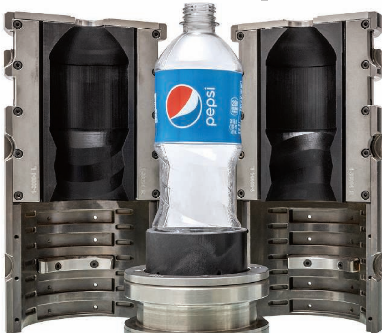
PepsiCo Inc. patented technology in late 2021 for a blow molding process that uses 3D printed mold inserts instead of metal tooling to create new bottle designs at a faster rate and reduced cost.
